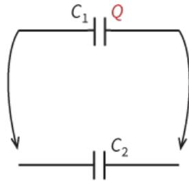
**Figure 23.16:** Capacitor of capacitance  $C_1$  is charged and then connected across  $C_2$ .
