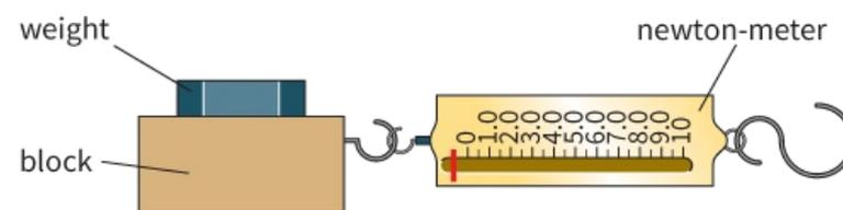
**Figure P1.17:** A newton-meter, just before it pulls a block along the bench. Look closely at Figure P1.17. When reading the meter, the uncertainty is the smallest scale division on the meter, unless one can reasonably read between the markings. This is difficult and so an uncertainty of 0.5 N, the smallest scale division, is reasonable.
