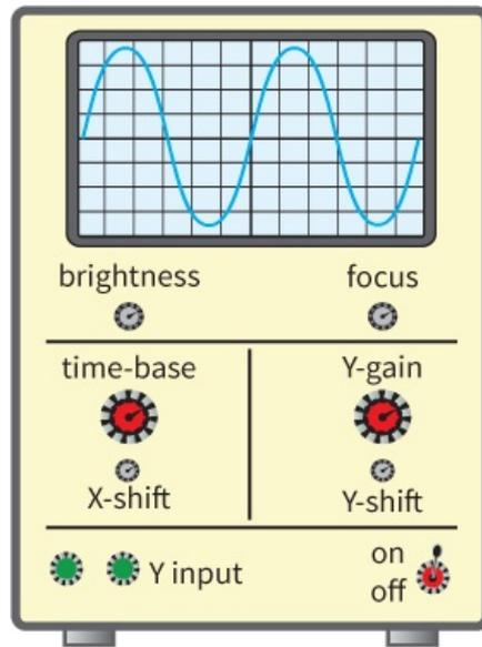
**Figure 27.6:** The controls of a typical CRO.
