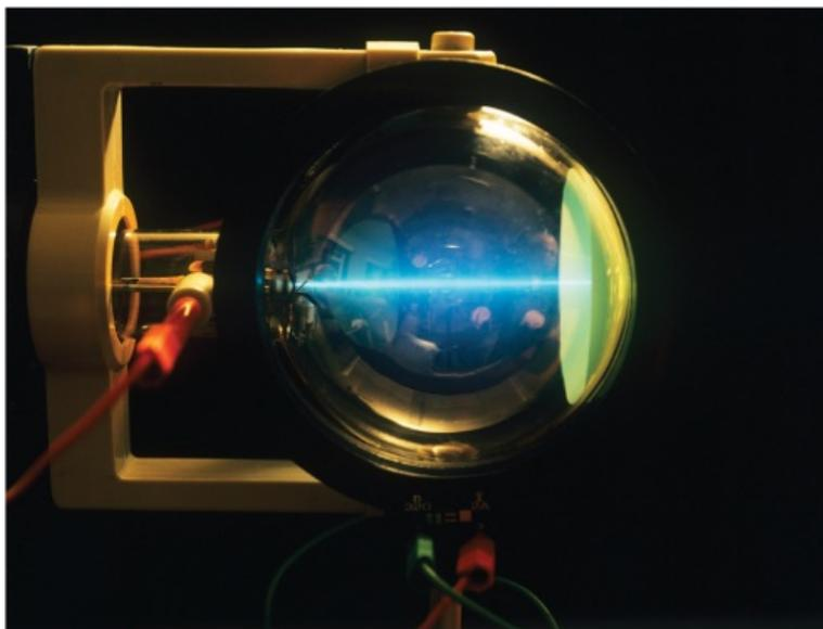
**Figure 25.2:** An electron beam tube.
