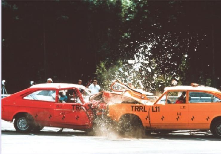
**Figure 6.1:** A high-speed photograph of a crash test. The cars collide head-on at  $15 \text{ m s}^{-1}$  with dummies as drivers.
