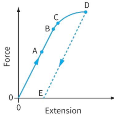
**Figure 7.9:** Force–extension graph for a wire.
