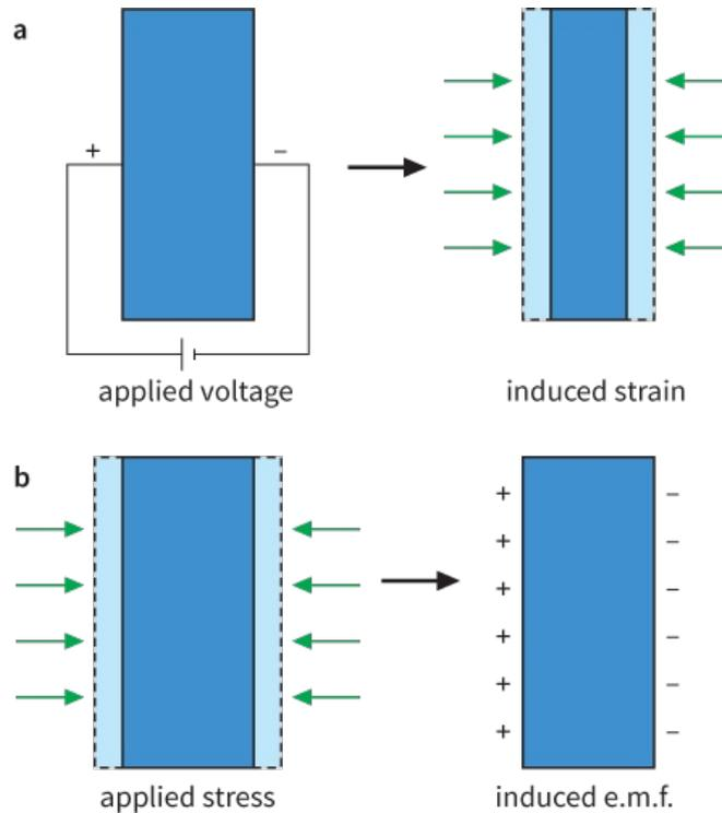
**Figure 30.13:** The **piezo-electric effect**. **a** An applied voltage causes a piezo-electric crystal to contract or expand. **b** An applied stress causes an induced e.m.f. across the crystal.
