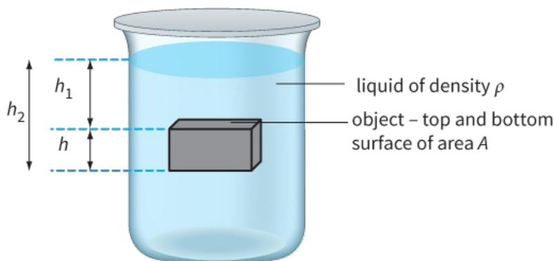
**Figure 7.4:** To explain Archimedes' principle.
