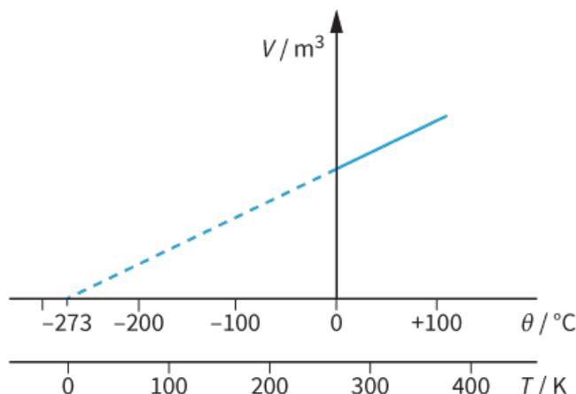
**Figure 20.6:** The volume of a gas decreases as its temperature decreases.
