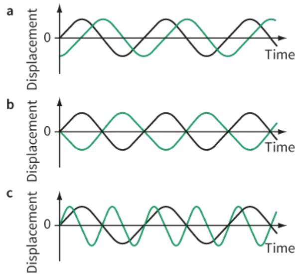
**Figure 18.9:** Illustrating the idea of phase difference.
