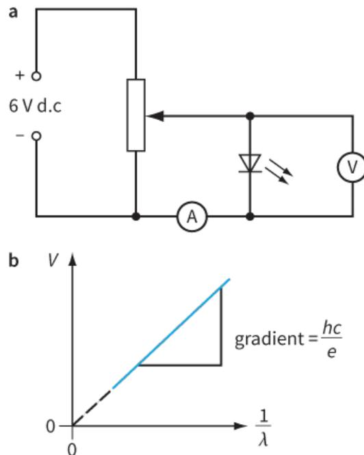
**Figure 28.6:** **a** A circuit to determine the threshold voltage required to make an LED conduct. An ammeter helps to show when this occurs. **b** The graph used to determine  $h$  from this experiment.
