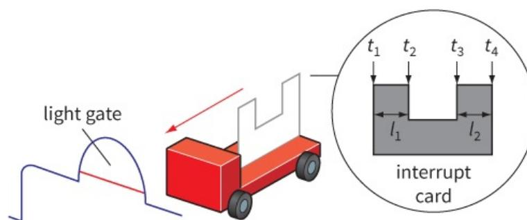
**Figure 2.8:** Determining acceleration using a single light gate.
