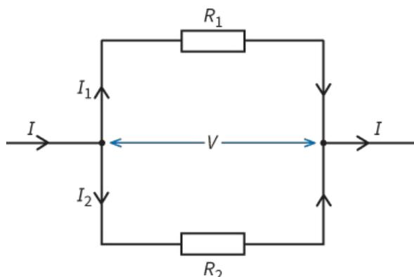
**Figure 9.18:** Resistors connected in parallel.
