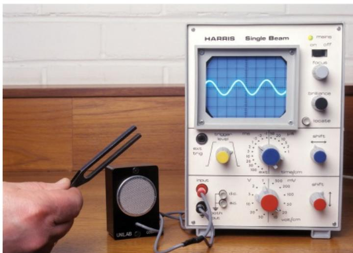
**Figure 12.6:** Determining the frequency of sound waves from a vibrating tuning fork.
