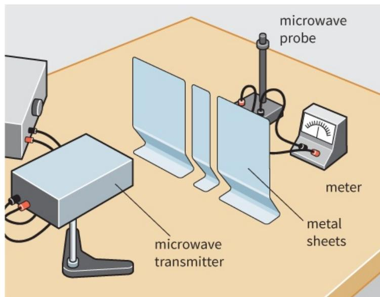
**Figure 13.17:** Microwaves also show interference effects.
