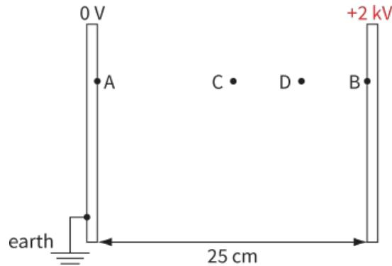
**Figure 21.16:** Two parallel, charged plates.
