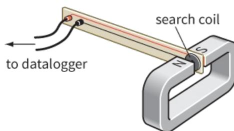
**Figure 26.18:** An e.m.f. is induced in the search coil when it is moved out of the field between the poles of the magnet. A search coil can be used to detect the presence of magnetic flux.
