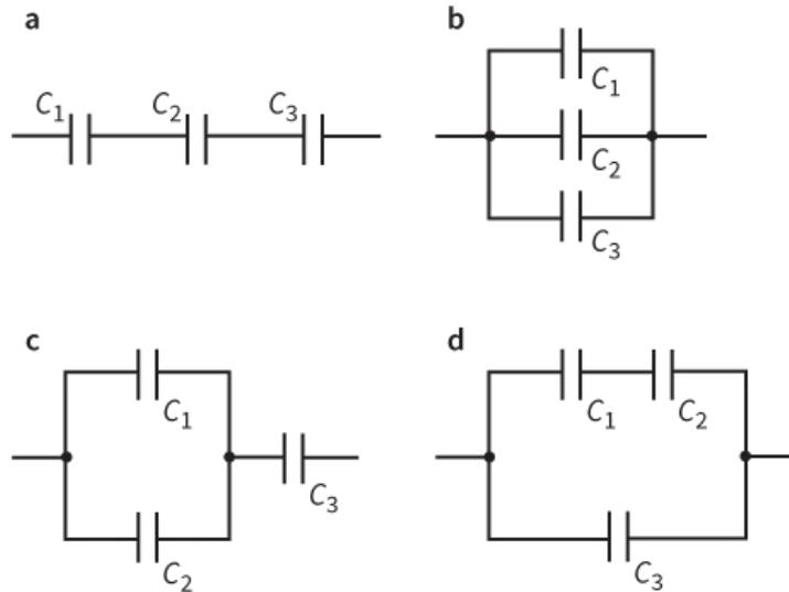
**Figure 23.14:** Four ways to connect three capacitors.
