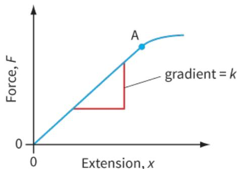
**Figure 7.8:** Force–extension graph for a spring.
