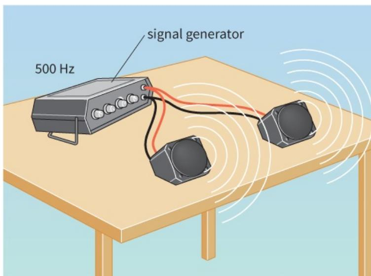
**Figure 13.11:** The sound waves from two loudspeakers combine to give an interference pattern. This experiment is best done outside so that reflections of sounds (or echoes) do not affect the results.
