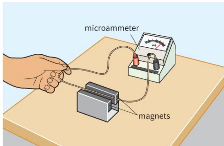
**Figure 26.4:** Investigating the current induced when a wire moves through a magnetic field.
