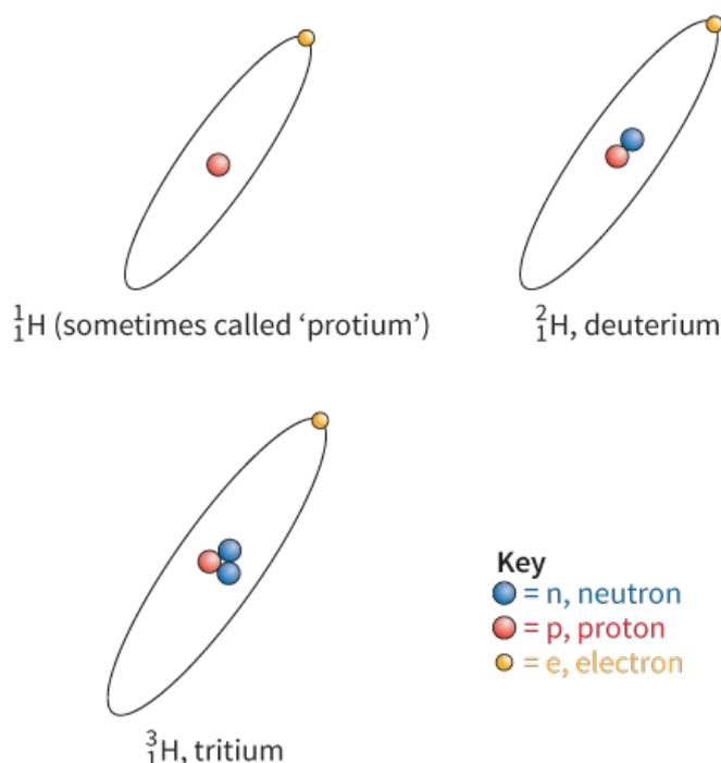
**Figure 15.7:** The isotopes of hydrogen.
