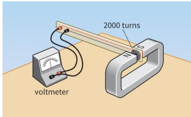
**Figure 26.19:** Using a search coil to determine the magnetic flux density of the field between the poles of this magnet.
