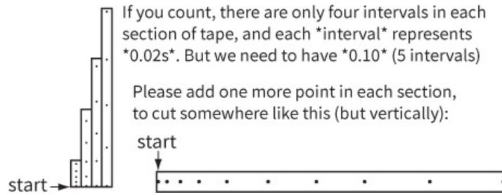
**Figure 2.9:** Ticker-tape for an accelerating trolley.
