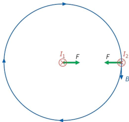
**Figure 24.23:** Explaining the force between two currents.
