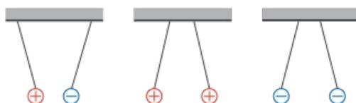
**Figure 21.2:** Attraction and repulsion between electric charges.
