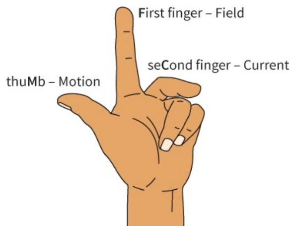
**Figure 24.9:** Fleming's left-hand (motor) rule.
