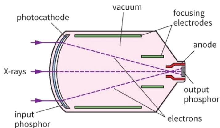
**Figure 30.6:** An X-ray image intensifier.
