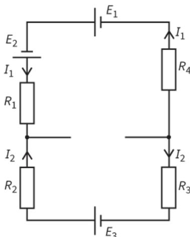
**Figure 9.12:** A loop extracted from a complicated circuit.
