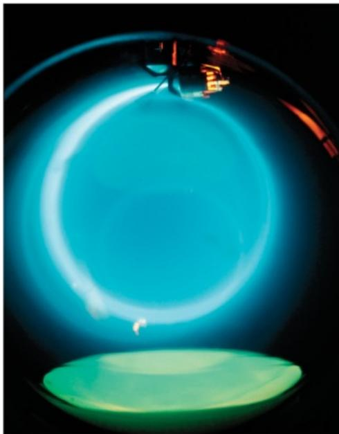
**Figure 25.8:** In this fine-beam tube, a beam of electrons is bent around into a circular orbit by a uniform magnetic field. The beam is shown up by the presence of a small amount of gas in the tube. (The electrons travel in an anticlockwise direction.)
