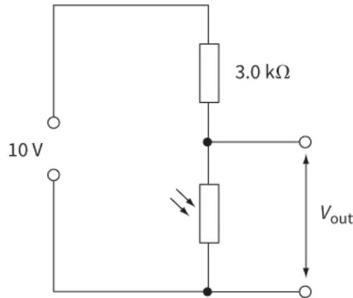
**Figure 11.8:** An LDR used as a sensor.
