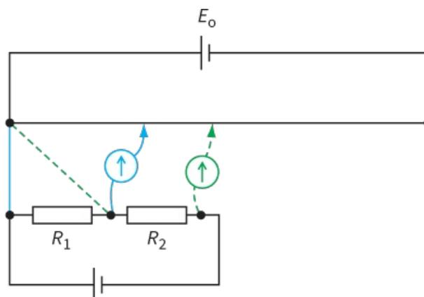
**Figure 11.13:** Comparing two potential differences using a potentiometer.
