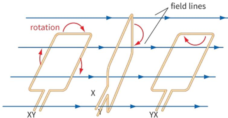
**Figure 26.25:** A coil rotating in a magnetic field.
