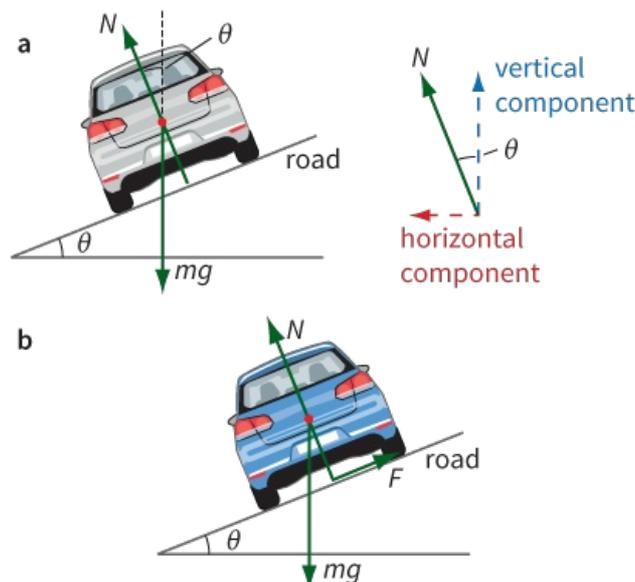
**Figure 16.14:** **a** On a banked road, the horizontal component of the normal contact force from the road can provide the centripetal force needed for cornering. **b** For a slow car, friction acts up the slope to stop it from sliding down.
