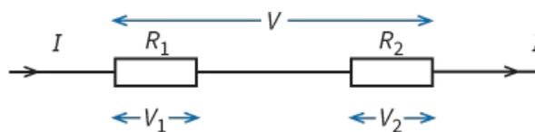
**Figure 9.16:** Resistors in series.
