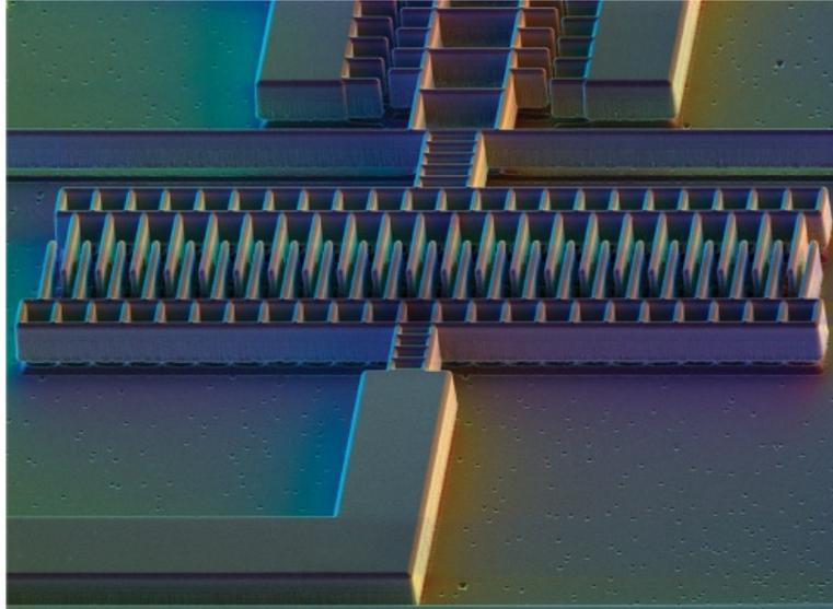
**Figure 2.7:** A micro-mechanical acceleration sensor is used to detect sudden accelerations and decelerations as a vehicle travels along the road. This electron microscope image shows the device magnified about 1000 times.
