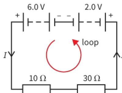
**Figure 9.9:** A circuit with two opposing batteries.
