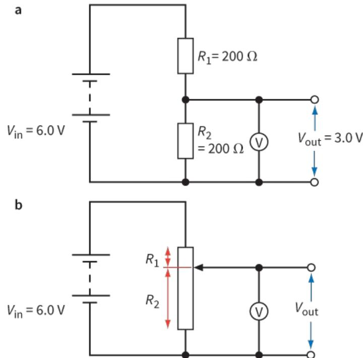
**Figure 11.6:** Two potential divider circuits.
