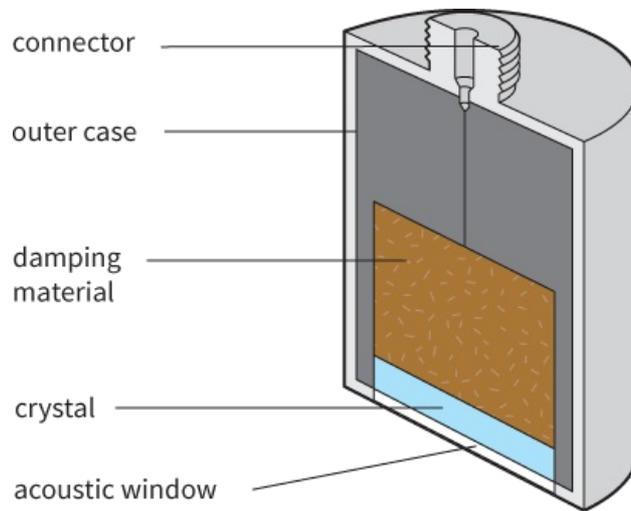
**Figure 30.14:** A section through an ultrasound transducer.
