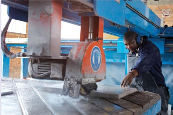
**Figure 13.1:** The headphones actively cancel out the noise - protecting the ears from damage.
