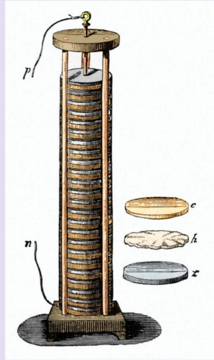
**Figure 11.1:** **a** Alessandro Volta demonstrating his newly invented pile (battery) to the French Emperor Napoleon. **b** Volta's pile, showing (top to bottom) discs of copper, wet felt and zinc.
