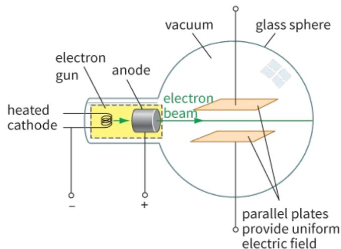
**Figure 25.4:** The construction of an electron beam tube.
