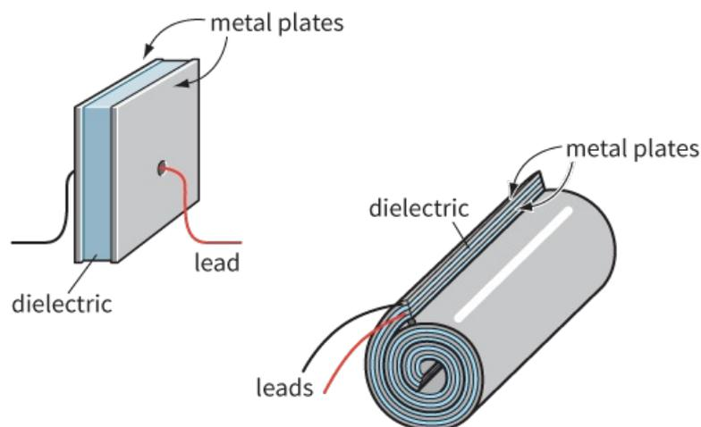
**Figure 23.3:** The construction of two types of capacitor.
