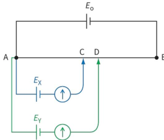
**Figure 11.12:** Comparing two e.m.f.s using a potentiometer.
