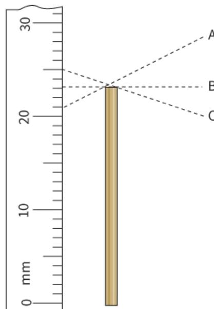
**Figure P1.2:** Parallax error.
