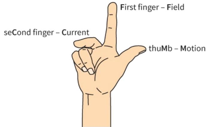
**Figure 26.8:** Fleming's right-hand (generator) rule.
