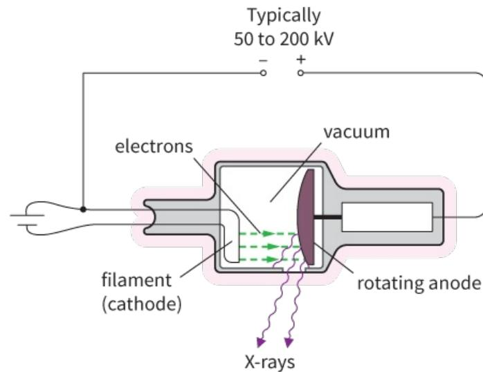
**Figure 30.4:** A simplified diagram of an X-ray tube.
