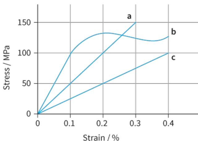
**Figure 7.15:** Stress-strain graphs for three materials.
