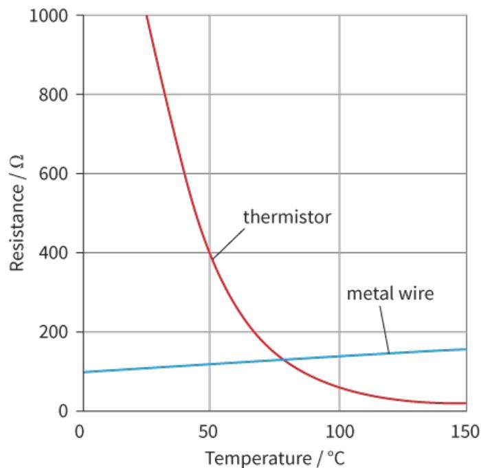
**Figure 11.10:** Variation of resistance with temperature.
