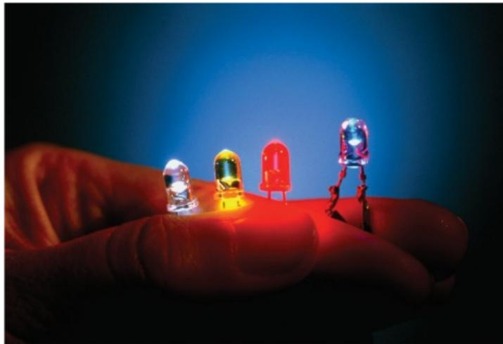
**Figure 28.5:** Light-emitting diodes (LEDs) come in different colours.
